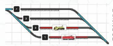
Detail from the Z21 schematic signal box of the Z21 app - when using the Z21 DETECTOR (10808) in addtion to the feedback message a picture of the locomotive is shown.
