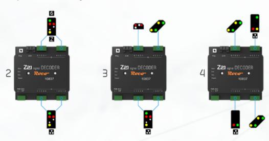
Depending on the complexity of the different signals, a varying number of devices can be connected.
